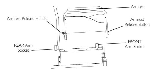
FIGURE 5.2 Removing/Installing Armrests
